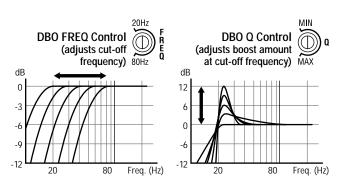
*Figure 9. Frequency response curves show range of Kappa 202a DBO controls.*
